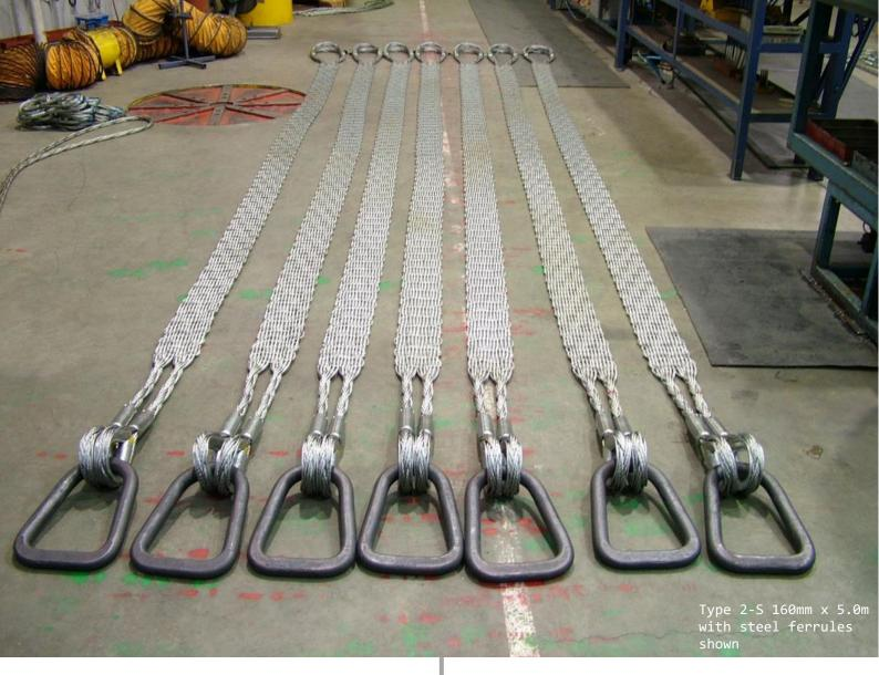
Flat Woven Steel slings manufactured by Andromeda are very flexible as I've seen them basketed close to capacity around steel beams with no kinks after use. Even FSWR slings basketed under moderate loads with packing around a steel beam shall get kinks and I would not consider using wire rope slings in the same way as they would be kinked even with edge protection in use.
