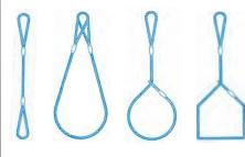
Suitable for straight, multi-leg, cradle and choker lifts to maximum cradle lift WLL of 55.7 tonnes.
