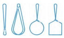
Suitable for straight, multi-leg, cradle and choker lifts to a maximum cradle lift WLL of 83.3 tonnes.
