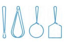
Strops suitable for straight, multi-leg, cradle and choker lifts to a maximum cradle lift WLL of 83.3 tonnes.
