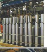
The ultimate choker lifting hot aluminium billets from casting beds leaving minimal marks compared to rigid grabs.
